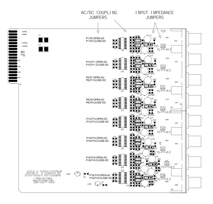
Note: In the diagram above, the jumpers are set for High impedance on the following ports: P20, P23, P21, P22, P24, P27, P25 and P26. (Jumpered pins have dark circles.)
